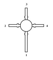
S872T Marking: S872T Plastic case ( $\sim$  TO 50) 1 = RF-output; 2 = Ground, 3 = RF-input, 4 = Ground
